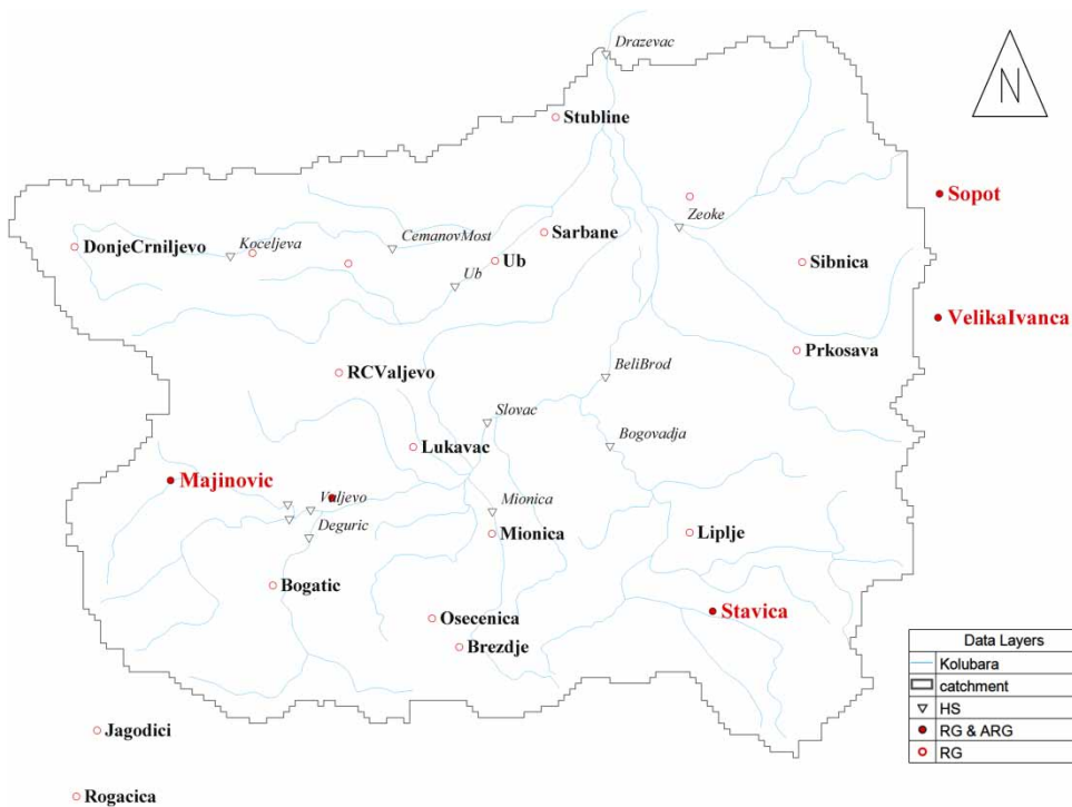
Figure 1 | The Kolubara River basin, locations of automatic rain gauges (filled circles), rain gauges (empty circles) and hydrologic stations (triangles).
