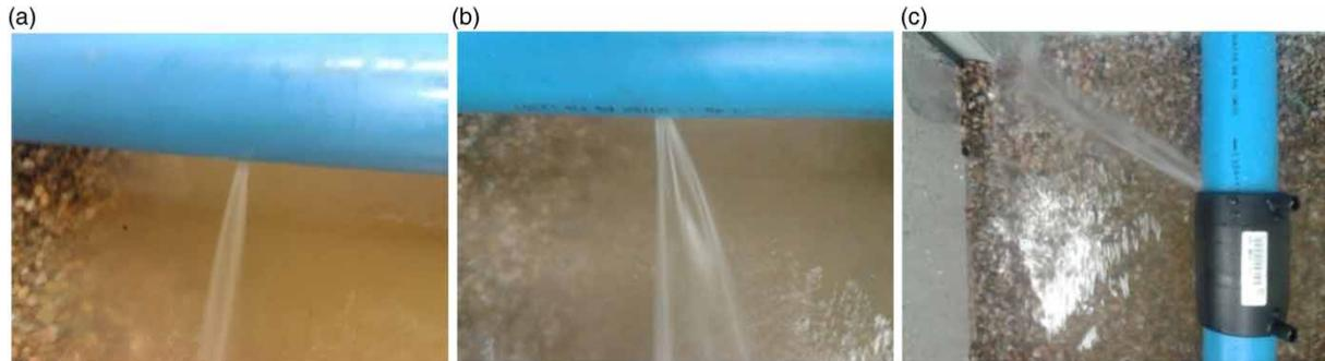
**Figure 3** | Photographs of leaks: (a) round hole; (b) longitudinal slit; (c) electrofusion joint.
