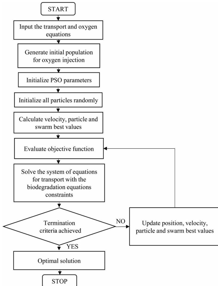
Figure 1 | Flow chart of PCM-BIO-PSO model.
