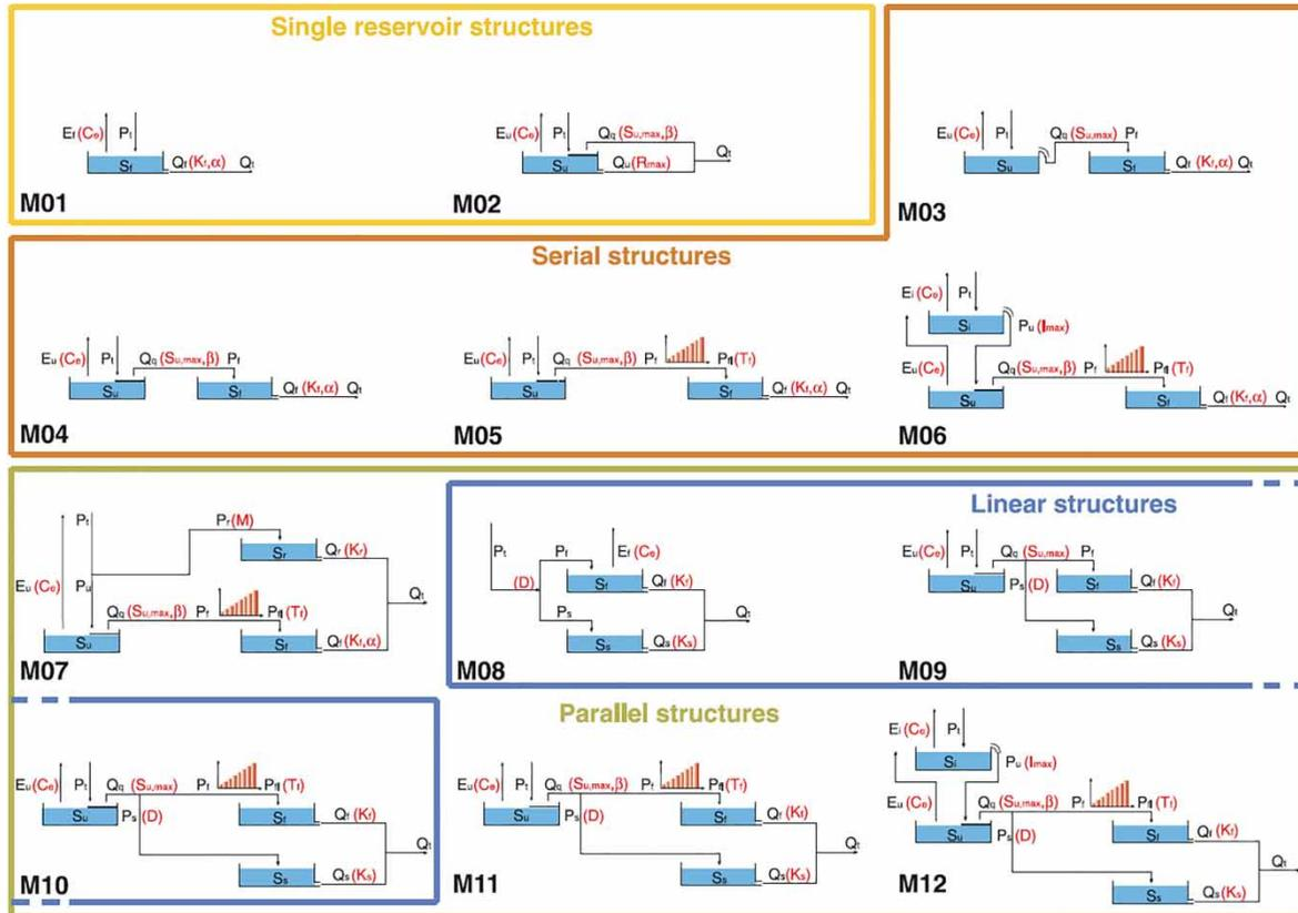
**Figure 1** | Twelve Superflex submodels considered in this study (Fenicia *et al.* 2014).  $P$ ,  $E$  and  $Q$  represent precipitation, potential evaporation and streamflow, respectively.  $S_i$ ,  $S_U$ ,  $S_R$ ,  $S_F$  and  $S_S$  represent storages of IR, UR zone, RR zone, fast reacting and slow reacting reservoirs, respectively.
