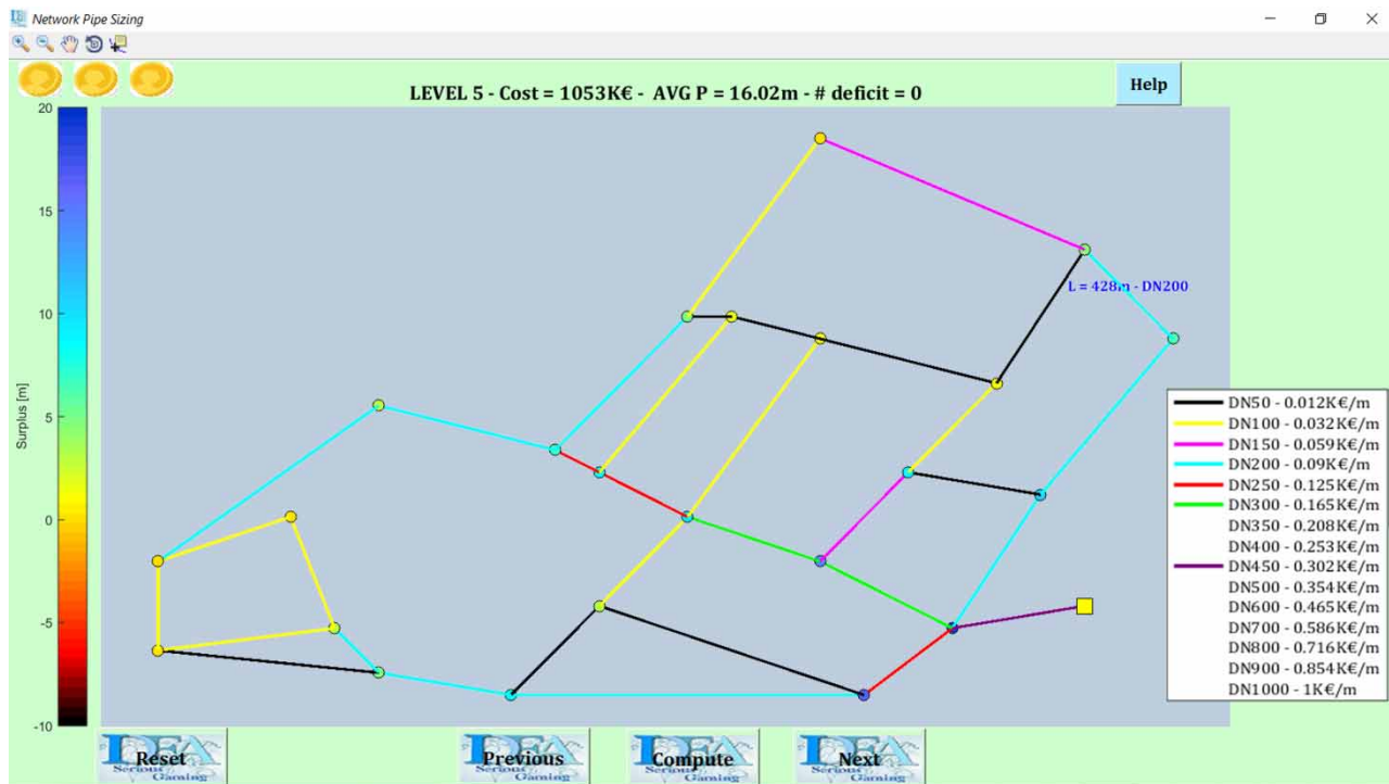
Figure 10 | Optimal solution screenshot of the fifth level of the NPS game for WDN sizing.
