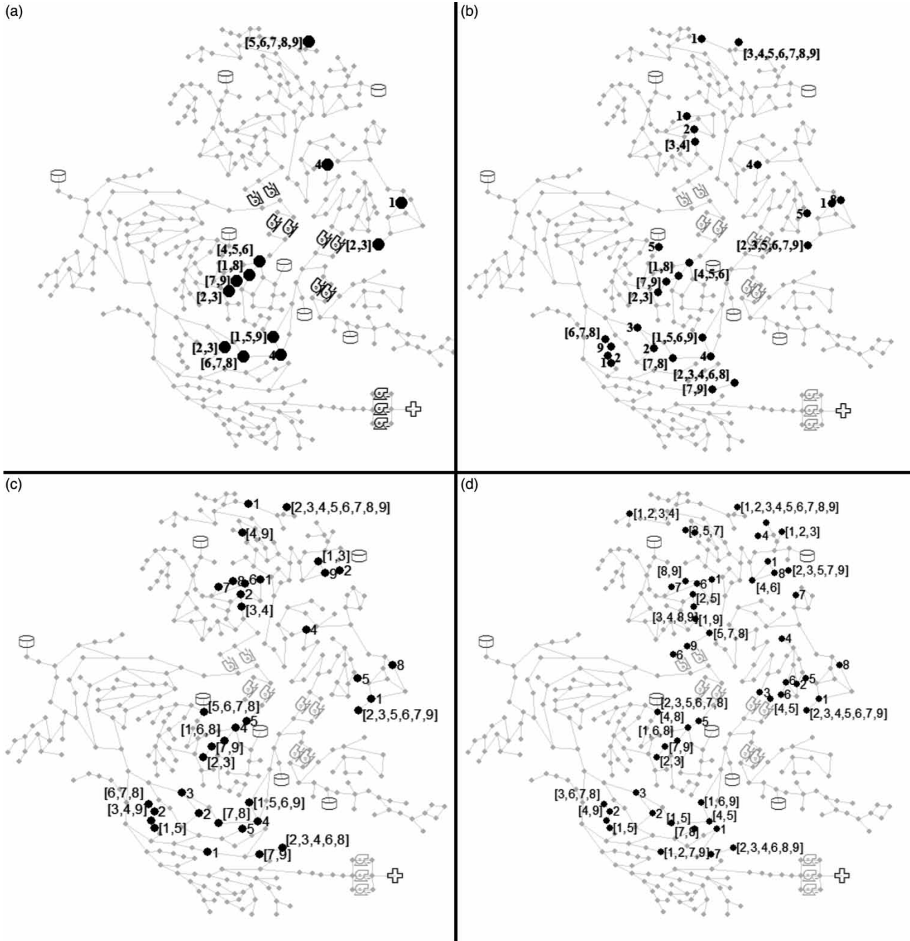
Figure 7 | The effect of device error on the location of pressure sensors. The solutions that have the ensemble size of (a) 3, (b) 6, (c) 8, (d) 15 sensors are selected from Figure 5. The number next to each sensor location corresponds to the error code. Error codes of 1, 2, ..., 9 represent 0.35, 0.4375, ..., 1.05 psi error thresholds, respectively.
