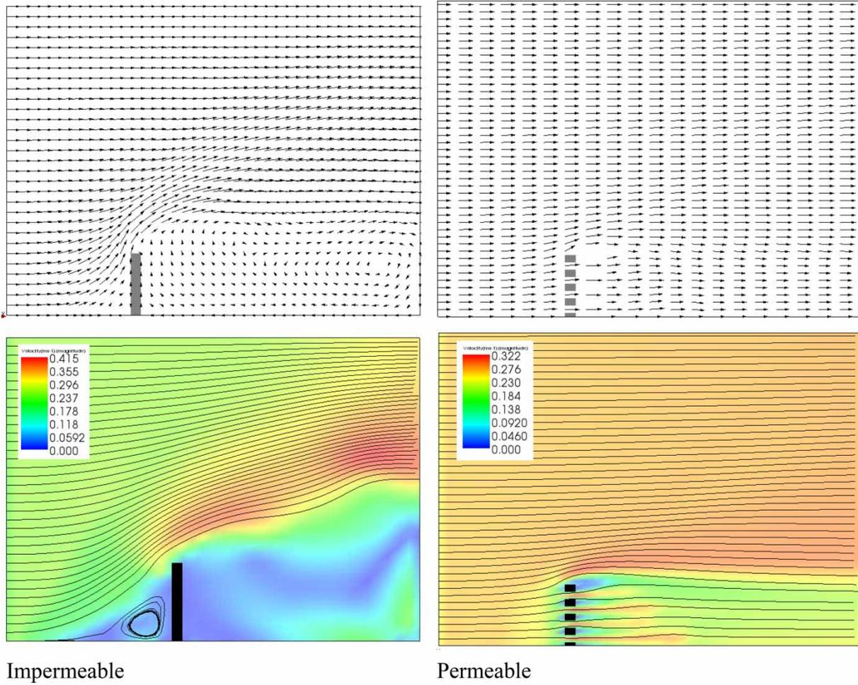
Figure 9 | Changes in flow pattern (streamlines and velocity vectors) due to permeability effect for  $P_r = 0.23$  and water depth 0.1 m.
