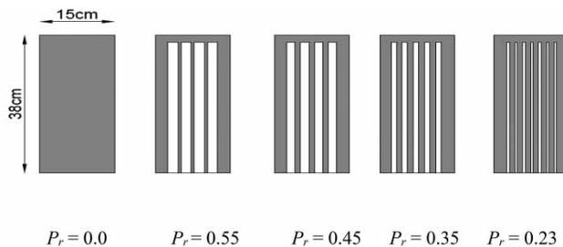
Figure 2 | Spur dike models of different opening ratios.
