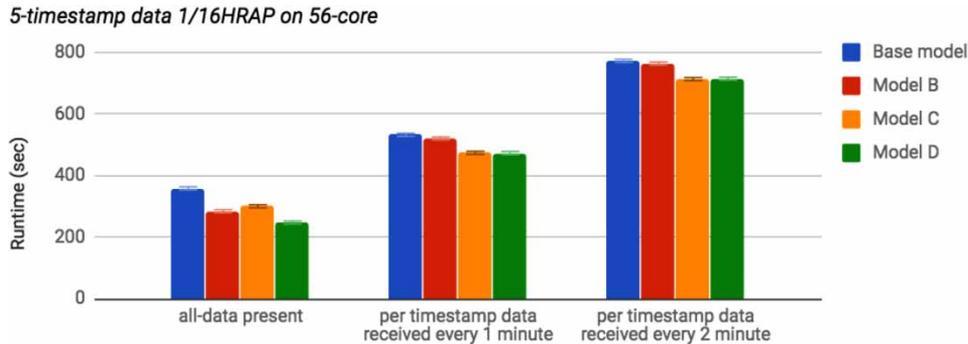
**Figure 7** | Runtime comparison among the different computing models with full parallelization when 5 min's worth of rainfall data is available all at once vs. when each min's worth is received in 1- or 2-min intervals.
