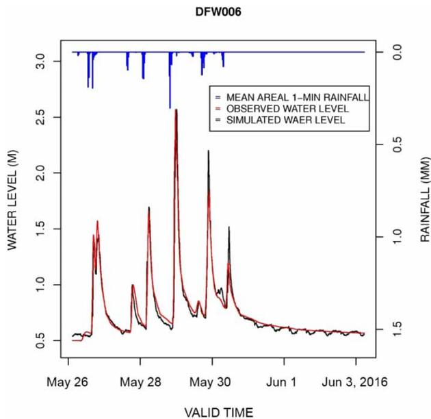
**Figure 2** | Example of the observed (black) vs. predicted (red) stage hydrographs and the associated hyetograph (blue) for a series of significant rainfall events in 26 May through 3 June 2016, at DFW006. Please refer to the online version of this paper to see this figure in color: <http://dx.doi:10.2166/hydro.2019.100>.
