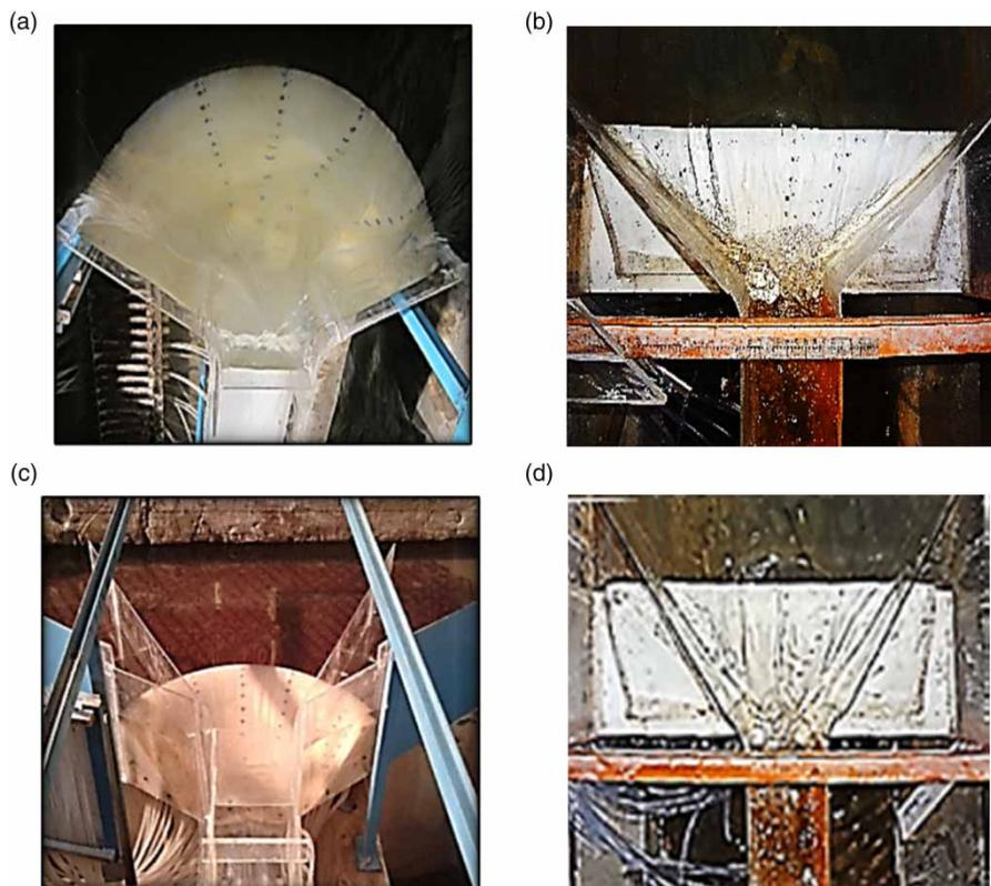
**Figure 2** | Photographs of the spillways with convergence angles of (a) 120° symmetric (curve axis), (b) 120° symmetric (straight axis), (c) 60° symmetric (curve axis), and (d) 60° asymmetric (straight axis).
