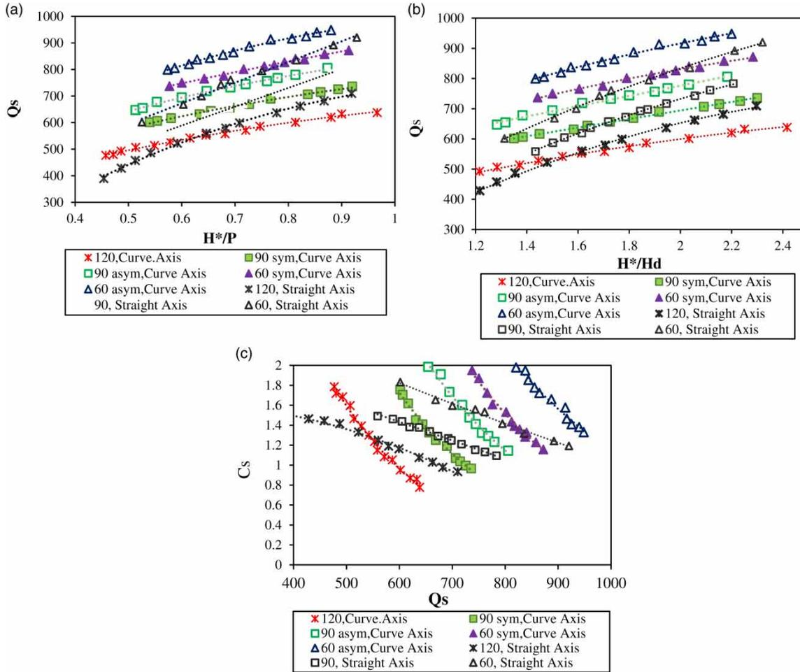
Figure 6 | Comparison of submerged discharge capacity of two physical models for varying  $\theta$  against (a)  $H^*/P$ , (b)  $H^*/H_d$ , and (c)  $C_s$ .
