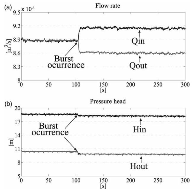
Figure 4 | Flow rate and pressure head at the ends of the pipeline (Experiment 1).
