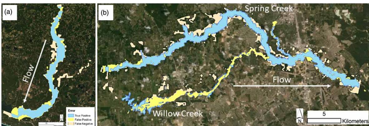
**Figure 3** | Spatial distribution of errors in the AutoRoute-simulated flood extent, including true positives (no error), false positives (model overestimates flood extent), and false negatives (model underestimates flood extent), for (a) Choctawhatchee River flood and (b) Spring and Willow creeks flood.
