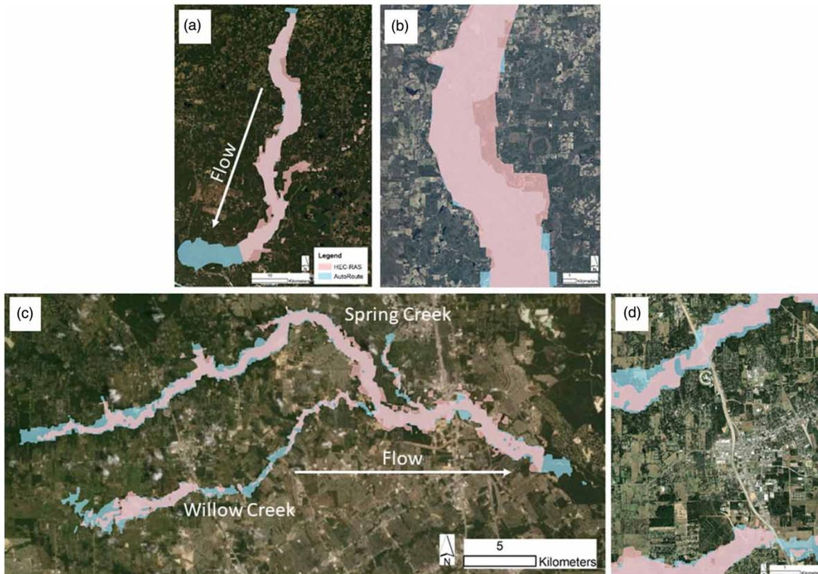
**Figure 4** | AutoRoute- and HEC-RAS-simulated flood-inundation extent for (a) Choctawhatchee River flood; (b) zoomed-in version of Choctawhatchee River flood; (c) Spring and Willow creeks flood; and (d) zoomed-in version of Spring and Willow creeks flood.
