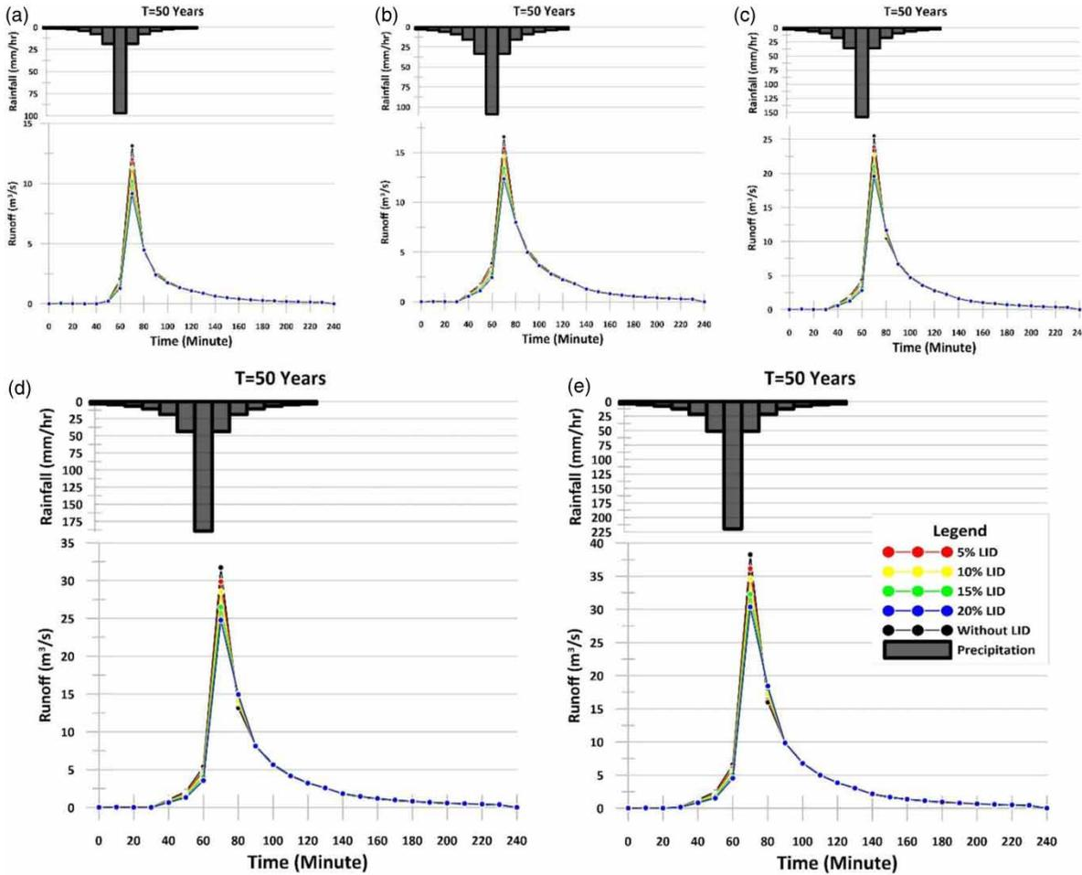
**Figure 8** | Hydrologic response of the catchment under land cover conversion scenarios and for each storm event. T = 2 years (a), T = 5 years (b), T = 10 years (c), T = 25 years (d), and T = 50 years (e).
