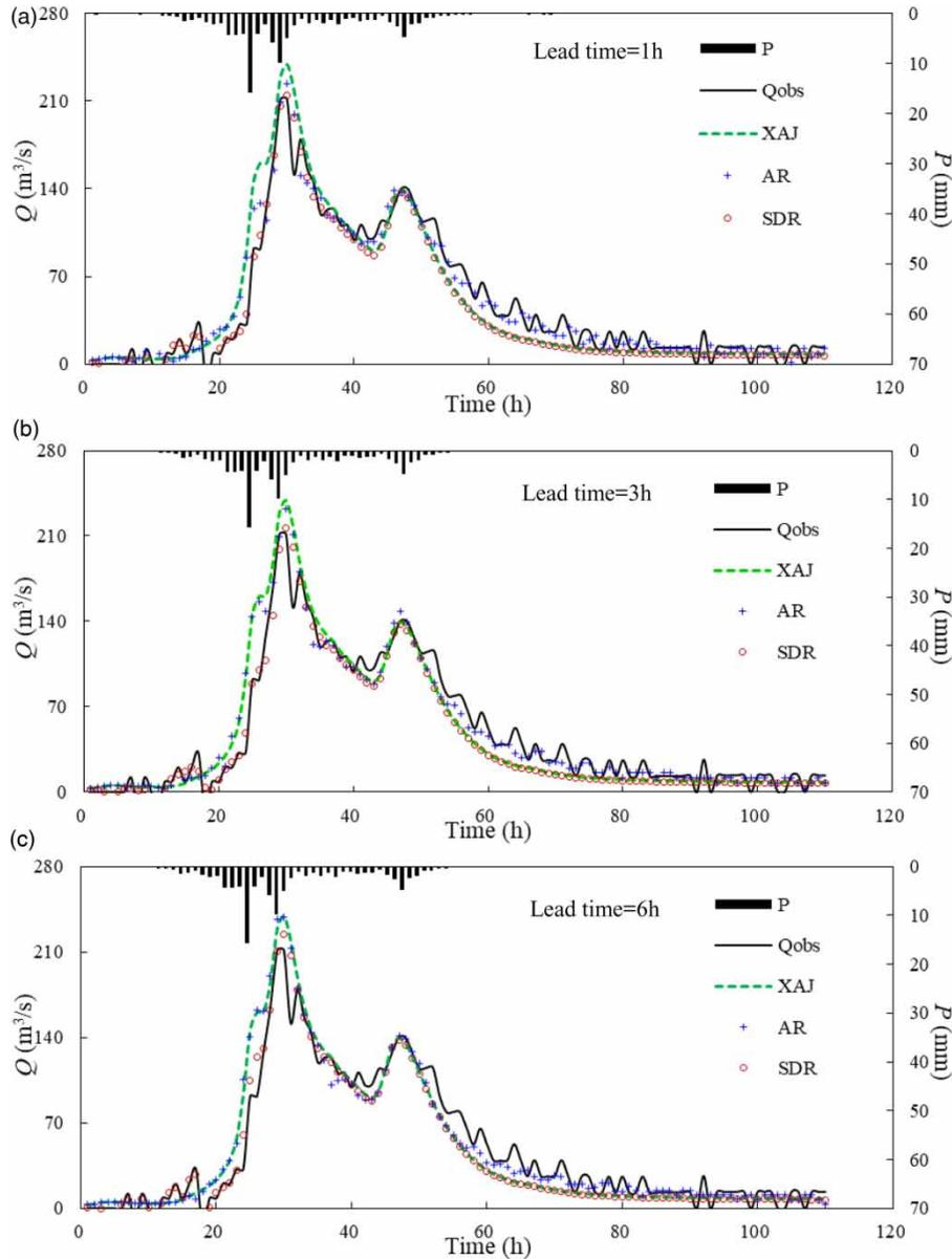
**Figure 7** | Hydrographs for the flood event 20071006 with different lead times in the BSK basin.
