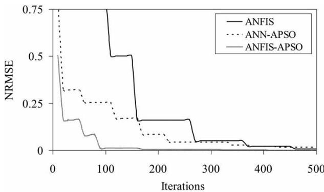
Figure 6 | Evolution of training NRMSE for different models versus the number of iterations in the estimation of air-water two-phase flow pressure loss coefficient.
