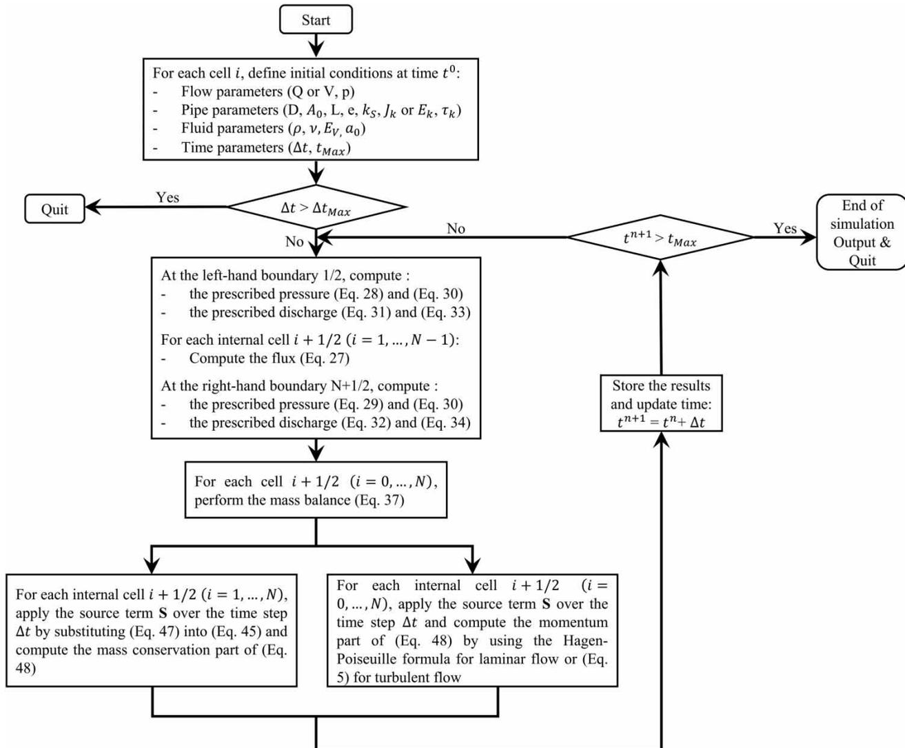
Figure 2 | Schematic of the proposed algorithm.
