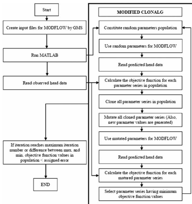
Figure 2 | The flow chart of the optimization model based on model calibration for groundwater modelling.
