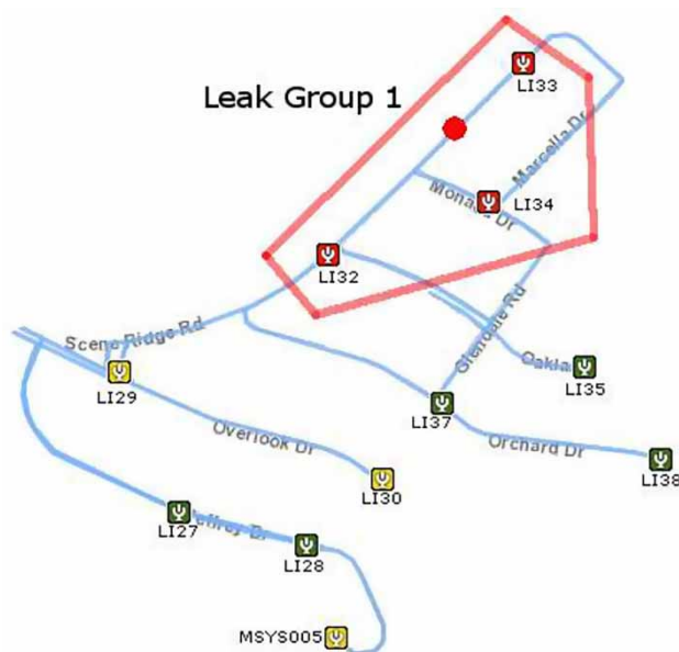
Figure 2 | Example of leak detection sensors deployed on a water pipe network. Please refer to the online version of this paper to see this figure in color: https://doi.org/10.2166/hydro.2021.093 .
