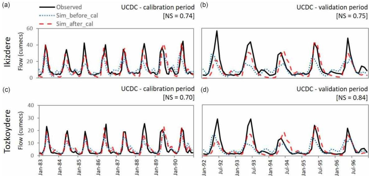
**Figure 6** | Observed flow comparison with simulated flow after calibration and validation (a) and (b) respectively for Ikizdere station; (c) and (d) for Tözköydere station (for UCDC – Tözköydere flow used before using Ikizdere for model optimization).
