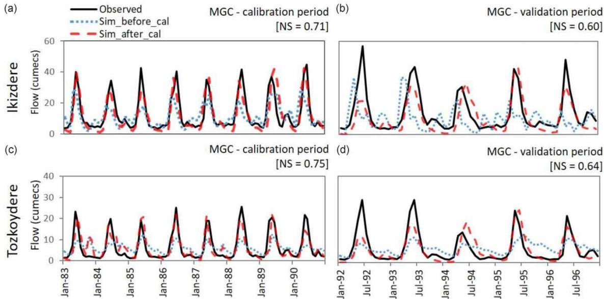
**Figure 5** | Observed flow comparison with simulated flow after calibration and validation (a) and (b) respectively for Ikizdere station; (c) and (d) for Tozkoydere station (for MGC – both Ikizdere and Tozkoydere flow used for model optimization).
