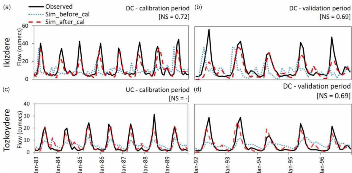
**Figure 3** | Observed flow comparison with simulated flow at Ikizdere station, for calibration and validation periods (a) and (b) respectively; and that of Tözköydere station validation (c) and (d) (for DC – only Ikizdere flow used for model optimization).
