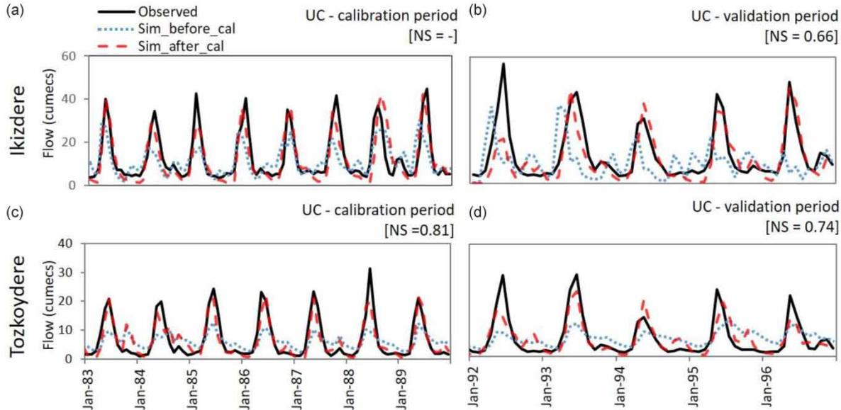
**Figure 4** | Observed flow comparison with simulated flow at Ikizdere station, for calibration and validation periods (a) and (b) respectively; and that of Tozkoydere station validation (c) and (d) respectively (for UC – only Tozkoydere flow used for model optimization).
