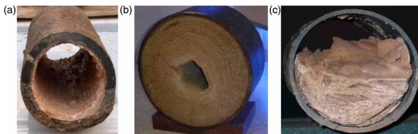
**Figure 1** | Pipe cross-section narrowing due to partial blockage features for metallic pipes: (a) and (b) diameter decrease caused by the regular deposit of sediment on the inner walls; for polymeric pipes: (c) accumulation on the lower part of the pipe section of material detached from the walls (Alegre & Covas 2010).
