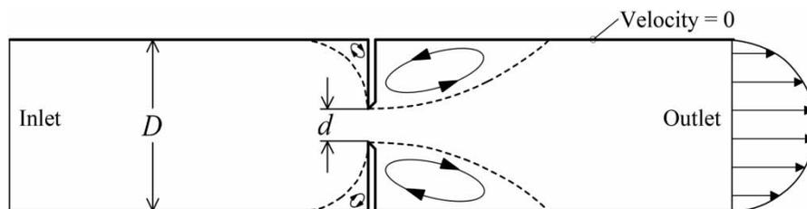
Figure 4 | Setup configuration.
