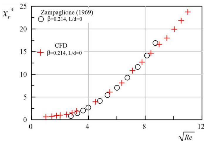
Figure 8 | Relative length of the expansion cone as a function of  $Re$  by Zampaglione (1969) vs. CFD results.
