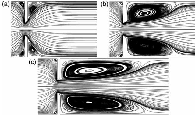
Figure 9 | CFD streamlines for  $\beta = 0.214$ : (a)  $Re = 1$ , (b)  $Re = 6$  and (c)  $Re = 10$ .
