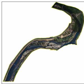
Step 4: Color the margin white and cut the orthophoto
