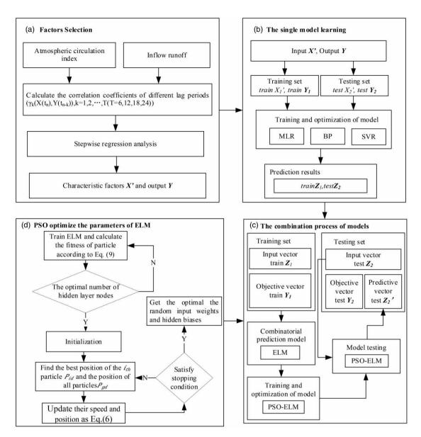
Figure 1 | Flowchart of the proposed combined model.
