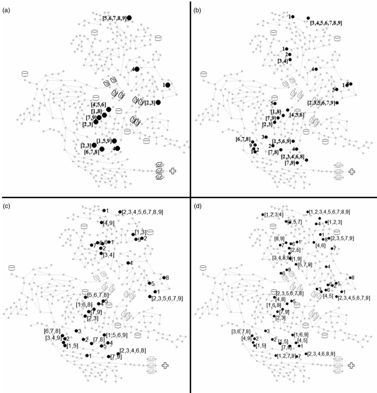
Figure 6 | Leak event coverage using the ensemble of ten-pressure sensors, which are selected from the trade-off for 0.7 psi error threshold when the leak event start time is (a) Scenario 1, (b) Scenario 2, (c) Scenario 3, and (d) Scenario 4. The map shows the number of sensors that detects a leak at that node. The shade represents the number of sensors (out of ten) that detects the leak event that is started at a node.
