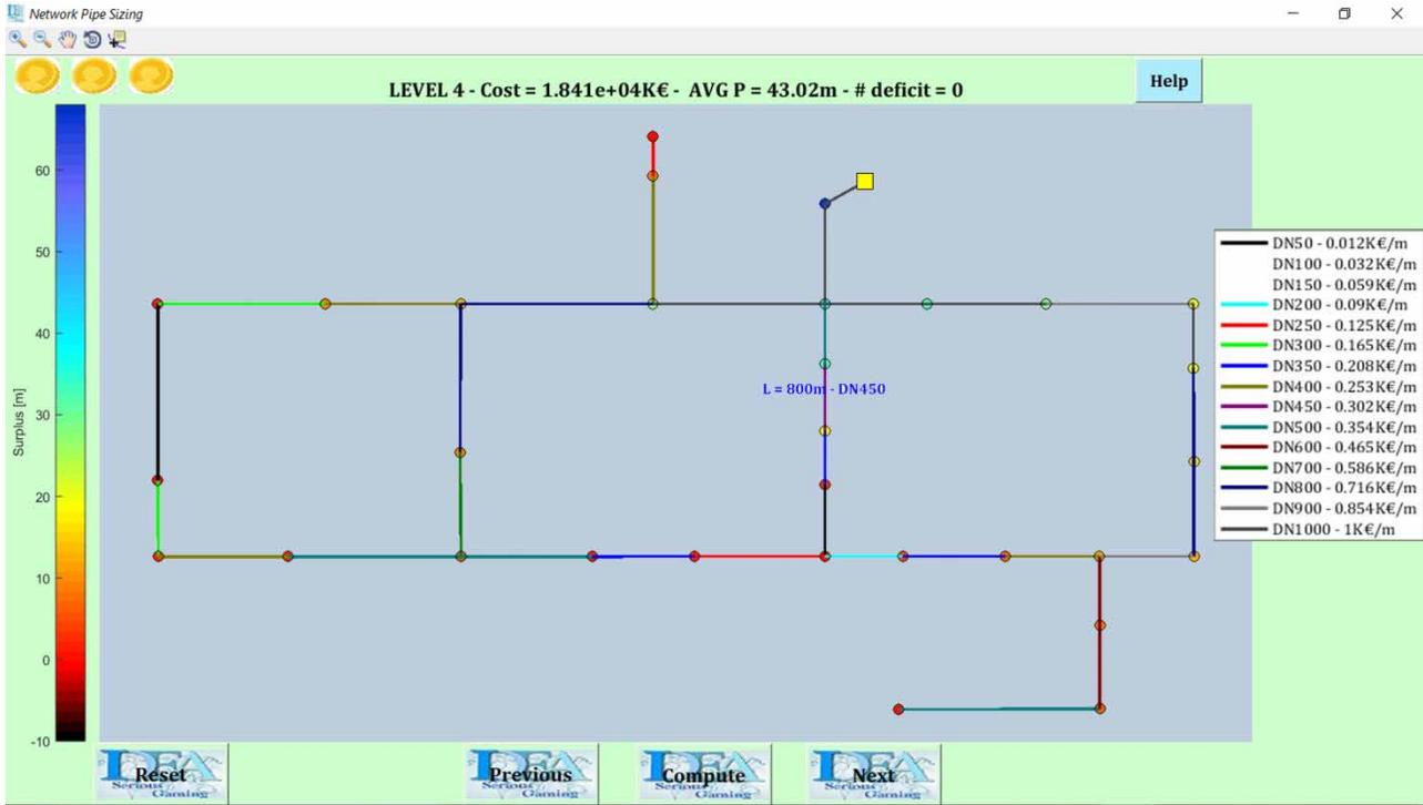
Figure 7 | Optimal solution screenshot of the fourth level of the NPS game for WDNs sizing.
