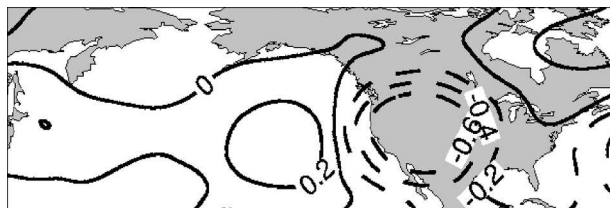
FIG. 9. Correlations between the mean Julian date (averaged for 84 sites in the western United States) when 50% of annual runoff occurs (CMD) and mean AMJJ 700-hPa heights. The solid lines indicate positive correlations, and the dashed lines indicate negative correlations. The contour interval is 0.2 and the first solid isoline is the zero correlation isoline.
