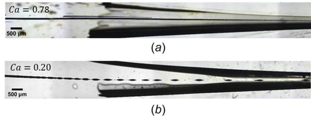
Fig. 11 Continuous mode (a) and dripping mode (b)
