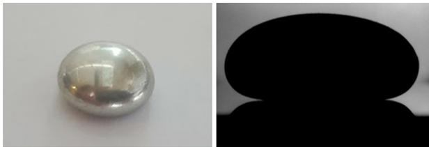
Fig. 9 A solidified Sn droplet after removing the PES for contact angle measurements
