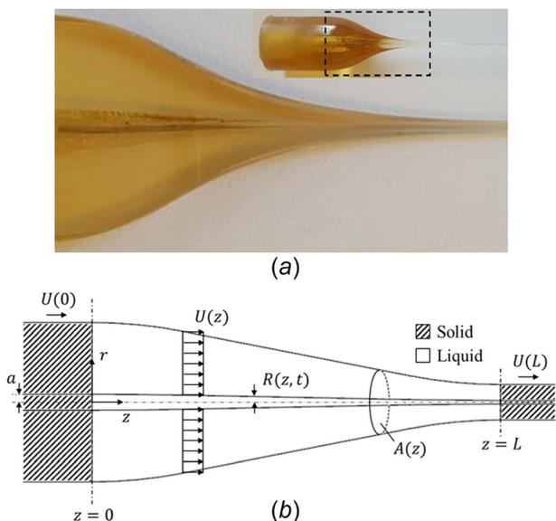
**Fig. 2** Image of the neck-down region (a) and the schematic (b) corresponding to an axisymmetric free surface extensional flow in the cladding entraining an immiscible molten metal from a nozzle (or melt front) located at  $z = 0$ . The entrained molten metal core has radius  $R(z, t)$ . Downstream at  $z = L$ , the metal solidifies with diameter  $R(L, t)$ .
