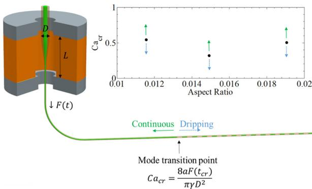
Fig. 10 Capillary number versus aspect ratio
