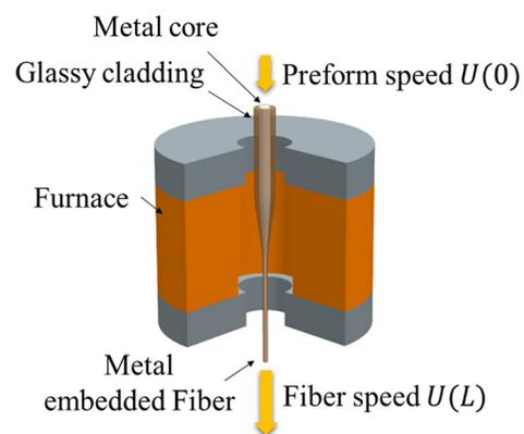
**Fig. 1 Schematic and process parameters of metal core fiber drawing from a preform**
