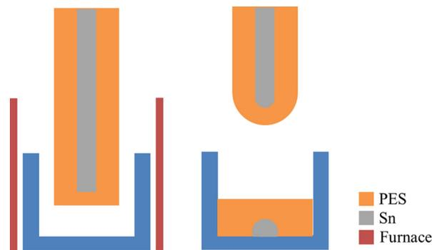
Fig. 7 Schematic of the procedure to obtain a Sn sessile drop surrounded by PES
