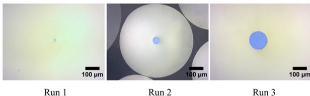
**Fig. 3 Cross-sectional images of the metal core fibers obtained from process parameters given in Table 2**
