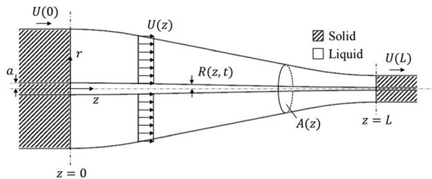
**Fig. 12** An axisymmetric free surface extensional flow  $(-(r/2)(dU(z)/dz), 0, U(z))$  in the cladding entrains an immiscible molten metal from a nozzle (or melt front) located at  $z = 0$ . The entrained molten metal core has radius  $R(z, t)$ . Downstream at  $z = L$ , the metal solidifies with diameter  $R(L, t)$ .
