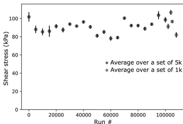
**Fig. 4** Durability over 100,000 cycles with a compression molded adhesive patch. The adhesive is loaded to 85% of its initial maximum shear stress, relaxed, and repeated for batches of 5000 cycles. After each batch of 5000 cycles the adhesive is manually repositioned and aligned.
