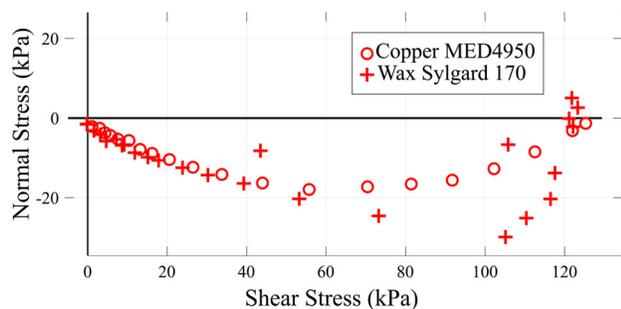
**Fig. 3** Empirical limit curves show maximum combinations of normal and shear stress before failure (by detachment or slipping). Circles show results for compression-molded NuSil MED 4950 in a copper plated mold [23]; plus symbols show corresponding results for Sylgard 170 from a wax mold, created as described in Ref. [20].
