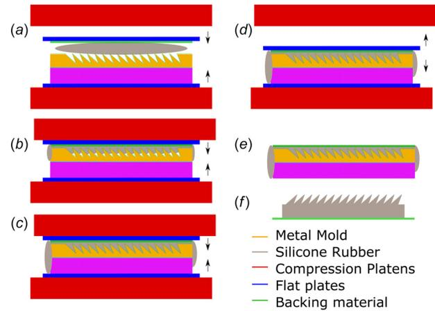
**Fig. 2 Flow diagram showing the steps of hot compression molding with metal molds. The steps (A–F) are described in Sec. 2.1.**
