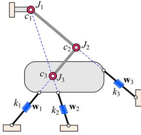
**Fig. 5 Dual elastic mechanisms in parallel and serial construction. The triangle formed by the three spring axes in the parallel mechanism is coincident with the triangle formed by the three joints in the serial mechanism.**
