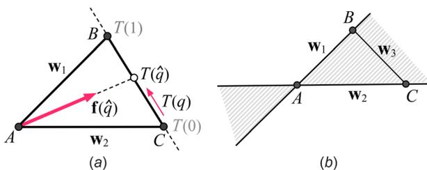
**Fig. 3** Location of center of elastic behavior: (a) if  $T(q)$  moves from  $C \rightarrow B$  along the finite segment  $CB$  as  $q$  varies  $0 \rightarrow 1$ , there must be a  $\hat{q}$  such that  $\mathbf{f}(\hat{q})$  passes points  $A$  and  $T(\hat{q})$  and (b) the center must be in the shaded area
