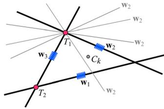
**Fig. 7** Realization of a planar stiffness with a parallel mechanism. The first spring axis  $w_1$  can be arbitrarily selected. The second spring can be selected from the pencil of lines passing through point  $T_1$ . The third spring axis is determined by the line passing through the instantaneous centers of twists  $t_1$  and  $t_2$ ,  $T_1$  and  $T_2$ .
