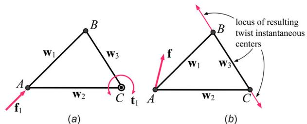
**Fig. 2 Force and resulting motion of a three-spring parallel mechanism: (a) a force along one spring axis results in a rotation about the opposite vertex of the triangle and (b) a force passing through one vertex results in a twist with an instantaneous center located on the line along the opposite side of the triangle**
