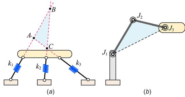
**Fig. 4** Location of stiffness center associated with a parallel and serial mechanism: (a) for a parallel mechanism, the center must lie within the triangle formed by the three spring axes and (b) for a serial mechanism, the center must lie within the triangle formed by the three joints
