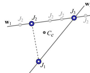
**Fig. 9** Realization of a planar compliance with a serial mechanism. The location of the first joint  $J_1$  can be arbitrarily selected. The second joint can be selected from any point on the line along wrench  $w_1$ . The third joint is determined by the intersection of the two lines along wrenches  $w_1$  and  $w_2$ .
