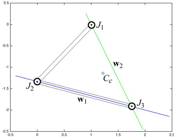
**Fig. 12 Synthesis of planar compliance with a serial mechanism. The location for each joint is identified based on its geometry. A serial mechanism can be constructed with three joints located at  $J_1$ ,  $J_2$ , and  $J_3$ .**
