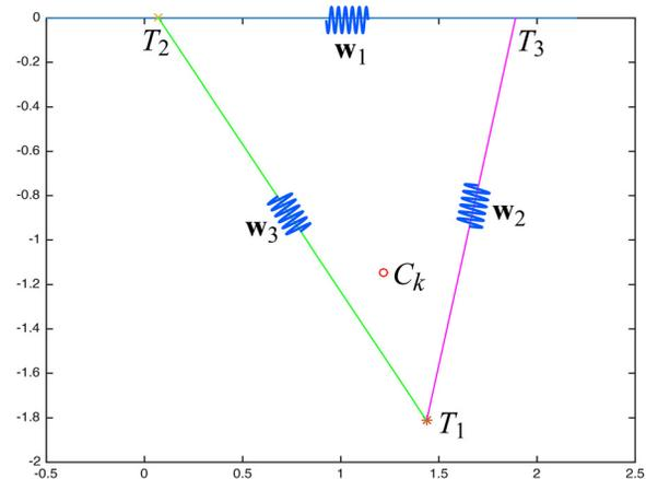
**Fig. 11 Synthesis of planar stiffness with a parallel mechanism.** The line of action for each spring is identified based on its geometry. A parallel mechanism can be constructed with three springs along the three spring wrenches  $w_1$ ,  $w_2$ , and  $w_3$ .
