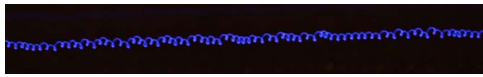
Fig. 5 A photographed trajectory illustrating period doubling and tripling. This is a trajectory of a somewhat more massive mechanism (1.7 g) with a larger displacement ( A \sim 0.5 mm), a frequency of 240 Hz and on cornmeal.
