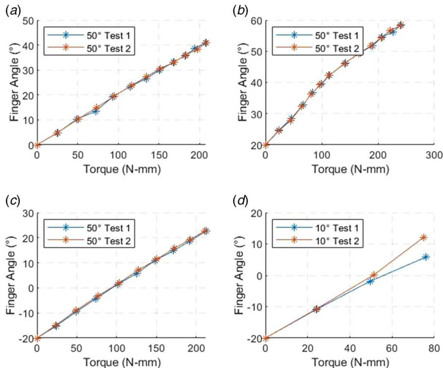
**Fig. 15 Lever mechanism results: (a) 50 deg stiffness position, 0 deg finger angle position, (b) 50 deg stiffness position, +20 deg finger angle position, (c) 50 deg stiffness position,  $-20$  deg finger angle position, and (d) 10 deg stiffness position, and 0 deg finger angle position**
