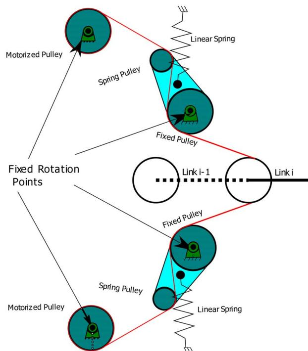
**Fig. 1** DLR's flexible antagonistic spring element design
