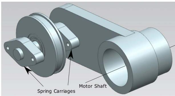
Fig. 11 Lever shaft assembly and spring carriage
