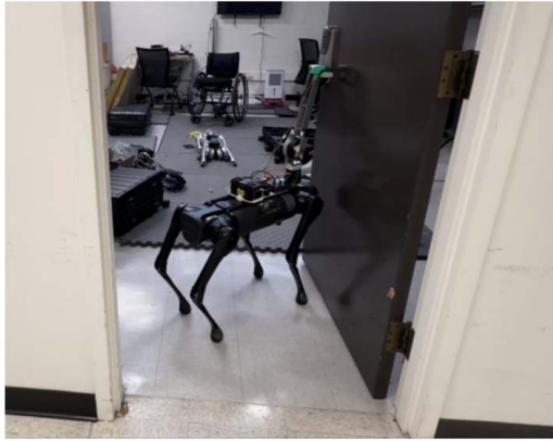
Fig. 9 Door opening using loco-manipulation MPC. In a hardware experiment, we were able to open a resistive door with manual commands.
