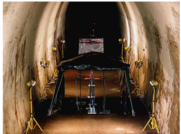
Figure 1. Elevated view of the setup for Experiment 1 (much of the foreground has been cropped to aid in viewing the apparatus). Two spatially separate arrays of LEDs can be seen (one for the 20-m observation distance and the other for the 40-m observation distance). The screen for the 20-m observation distance trials has been removed (although the canopy remains). While only two LEDs were turned on in each experimental trial (one central LED and one lateral LED), all of the LEDs were turned on for this demonstration. The lateral LEDs in each case were located exactly at the observation distance. The central LEDs could be at one of 7 different depths relative to these lateral LEDs. Several LEDs are occluded by the polyethylene screen or canopy in this view, but all were visible from the observer's vantage point.
