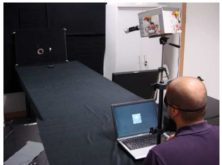
Figure A2. Experimental layout for the control experiments. The layout is photographed with normal room illumination. During experiments, normal room illumination was extinguished and stimuli were illuminated only by the pinpoint light source (upper right).
