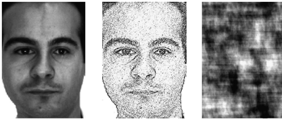
Figure 8. A grayscale image of a face (left), the same image with a randomly scrambled amplitude spectrum (middle), and the same image with a randomly scrambled phase spectrum (right).
