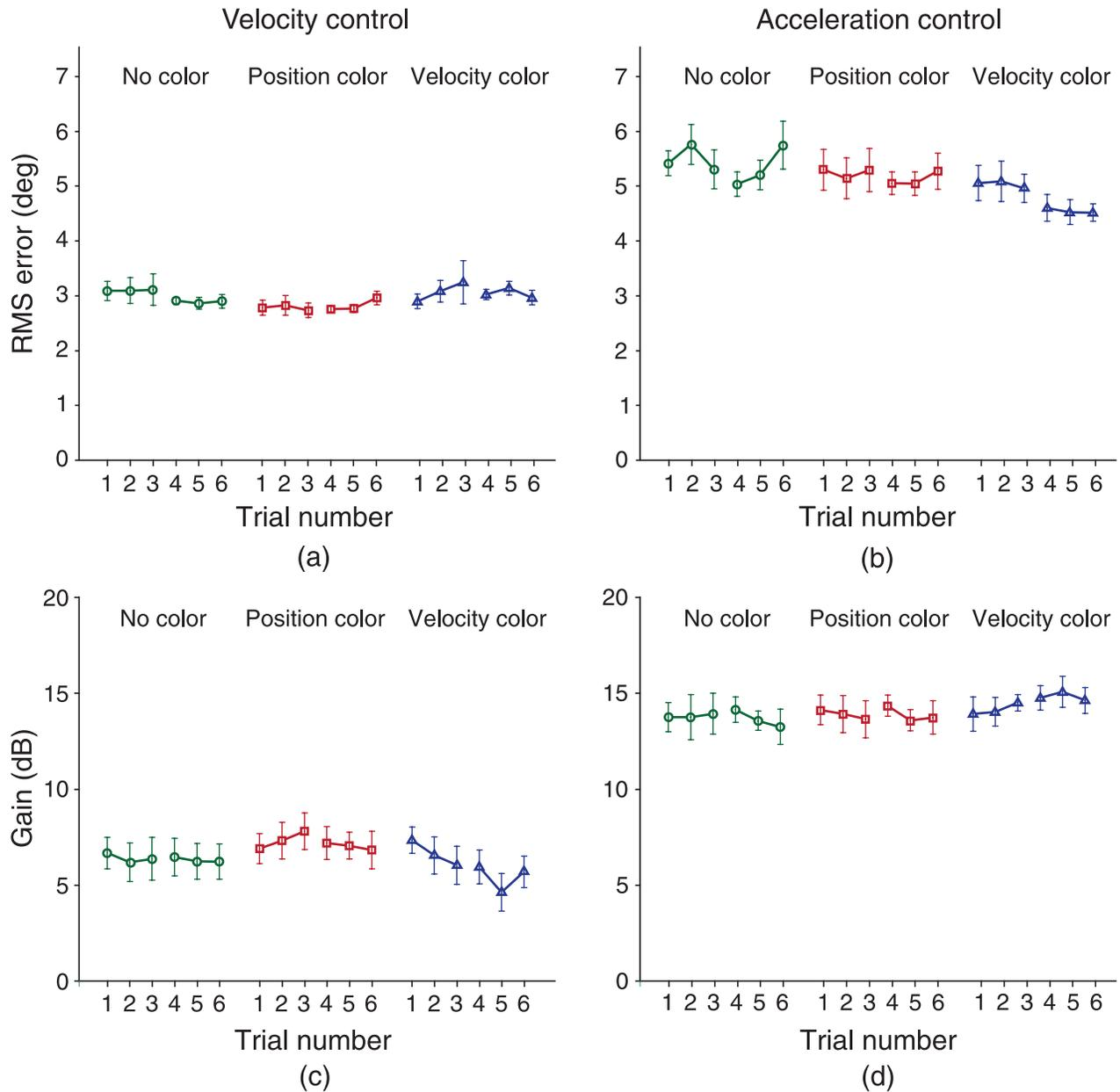
Figure 8. Mean RMS error against trial number for the three color-feedback conditions for (a) velocity control and (b) acceleration control. Mean gain against trial number for the three color-feedback conditions for (c) velocity control and (d) acceleration control. Error bars represent SEs across seven participants.
