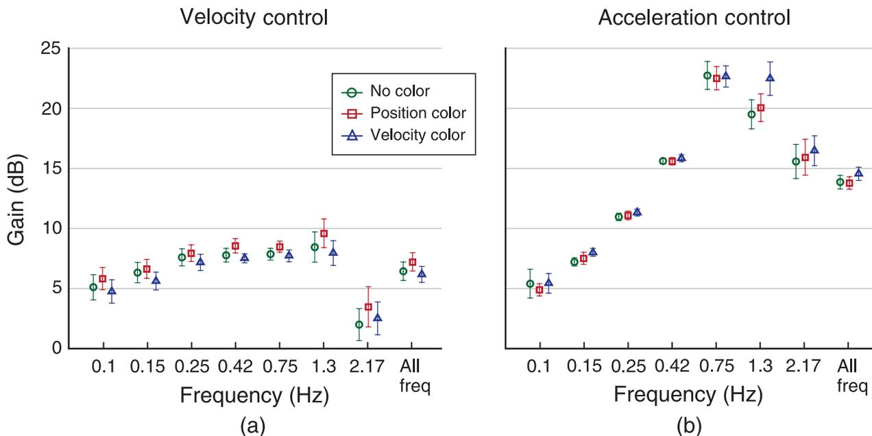
Figure 6. Mean gain of the human operator transfer function ( $Y_p$ ) against perturbation frequency for the three color-feedback conditions for (a) velocity control and (b) acceleration control. The rightmost points in the graphs plot the mean gain averaged across the seven frequencies. Error bars represent SEs across seven participants.
