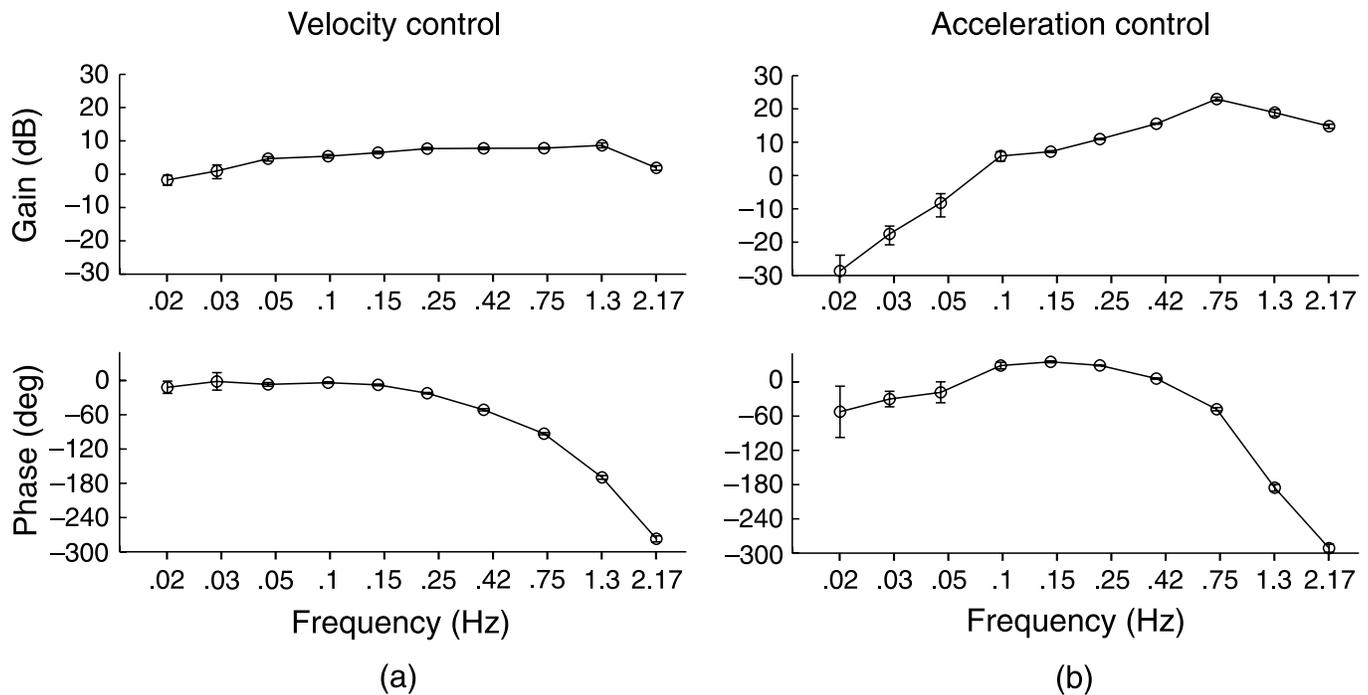
Figure 4. Frequency response (Bode) plots for the human operator transfer function ( $Y_p$ ) for the baseline no-color condition. The top panels depict mean gain and the bottom panels depict mean phase averaged across seven participants as a function of perturbation frequency for (a) velocity control and (b) acceleration control. Error bars represent SEs across participants (some of them are smaller than the data symbols).
