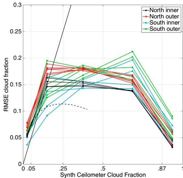
FIG. 6. The RMSE between the synthetic ceilometer observations and the 15-min averaged  $50^\circ$  TSI cloud fraction for each ceilometer cloud fraction class. Dashed line is from Eq. (10) in Berg and Stull (2002), while the solid line is a 1:1 fit; points above the solid line have a greater variability than the signal.
