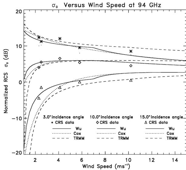
FIG. 10. The  $\sigma_o$  vs ocean surface wind speed at different incidence angles. Results from the quasi-specular scattering model are shown as the solid, dotted, and dashed lines.
