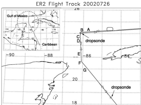
FIG. 7. ER-2 flight track on 26 Jul 2002. A larger-scope plot is shown at the upper left-hand corner. ER-2 flew the track on its outbound trip and on its return trip. It made turns at way points B and F.
