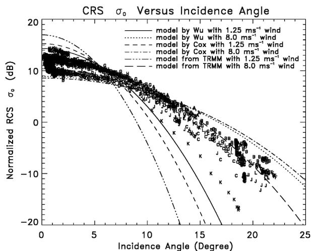
FIG. 9. The  $\sigma_o$  measured by the CRS vs incidence angle from different turns made in different days. A total of 12 turns from clear weather is shown.
