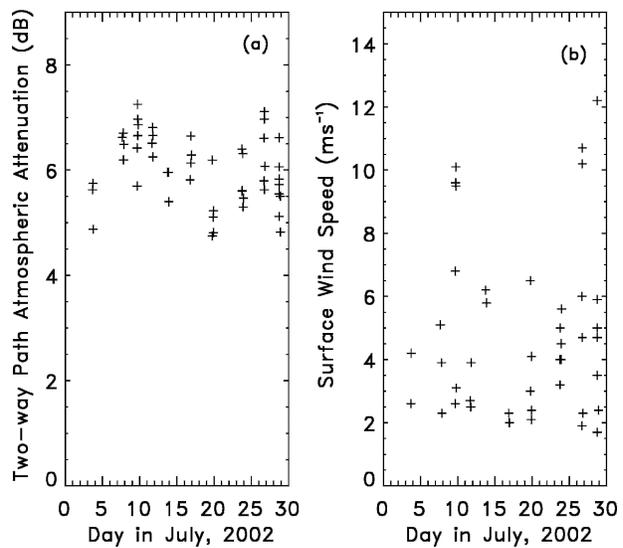
FIG. 4. (a) Two-way PIA due to water vapor and oxygen absorption at 94 GHz derived from dropsonde data collected from CRYSTAL-FACE. It shows the PIAs with a mean of 5.8 dB and a standard deviation of 0.65 dB. (b) Ocean surface wind speed measured by dropsondes during CRYSTAL-FACE.
