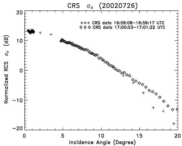
FIG. 11. The  $\sigma_o$  from a turn with a 100° heading change, which indicates that  $\sigma_o$  varies relative to wind direction for an incidence angle larger than 12°.
