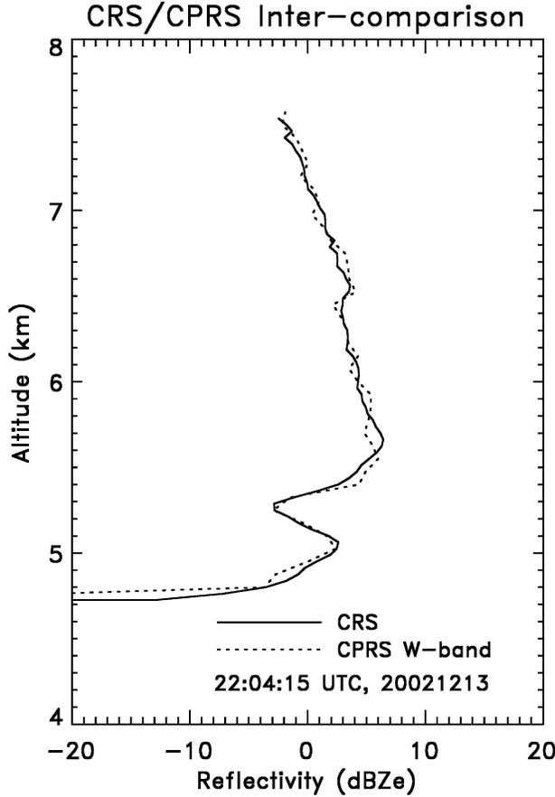
FIG. 1. CRS intercomparison with CPRS W-band radar at UMass, 13 Dec 2004. The mean difference between the two profiles is within 1 dB.
