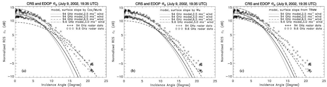
FIG. 6. The  $\sigma_o$  measured by the CRS vs incidence angle during the turn shown in Fig. 5, and compared to the quasi-specular model with 2.5, 3.0, and 6.0 m s<sup>-1</sup> wind speeds as well as using (a) Cox and Munk's (1954), (b) Wu's (1972, 1990), and (c) TRMM's surface slope relationships. For comparison, EDOP data and model predictions at 9.6 GHz and 3.0 m s<sup>-1</sup> wind are also shown in each figure.
