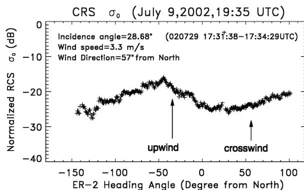
FIG. 12. The  $\sigma_o$  vs ER-2 heading angle.
