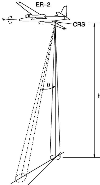
FIG. 2. Geometry of the CRS measurements from NASA ER-2 during CRYSTAL-FACE. The CRS was installed in a nadir-looking mode. The radar beam was scanned in a cross-track direction when ER-2 rolled its body to one side during turns.
