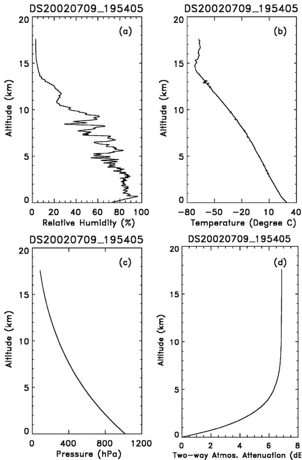
FIG. 3. Dropsonde measurements at 1954 UTC 9 Jul 2002: (a) relative humidity, (b) temperature, and (c) pressure. (d) The two-way cumulative path attenuation due to water vapor and oxygen absorption at 94 GHz.
