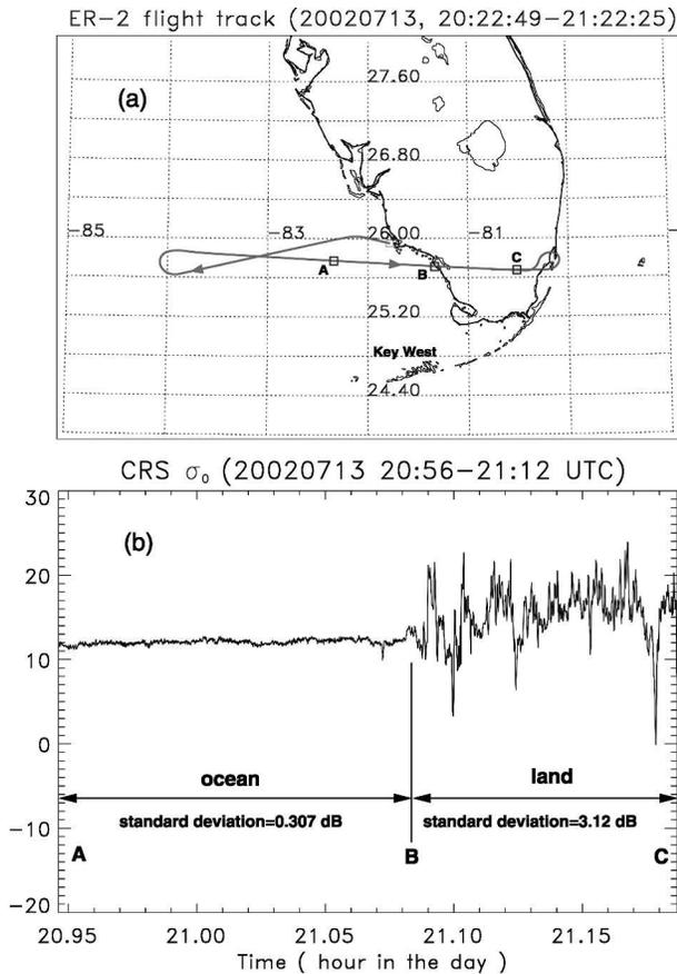
FIG. 13. (a) ER-2 flight track on 13 Jul 2002, which crossed the coastline at point B (2104:53 UTC). (b) The  $\sigma_o$  measured by the CRS from 2056 to 2112 UTC. From the ocean to inland, it shows significant increase in the standard deviation of  $\sigma_o$ .
