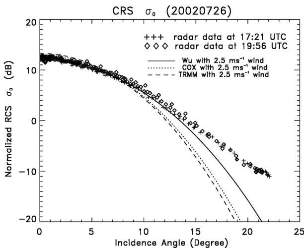
FIG. 8. The  $\sigma_o$  measured by the CRS vs incidence angle from the turns near way point F shown in Fig. 7. Crosses represent measurements from the outbound turn through E, F, and G consequentially. Diamonds represent measurements from the turn through G, F, and E on the return trip consequentially.
