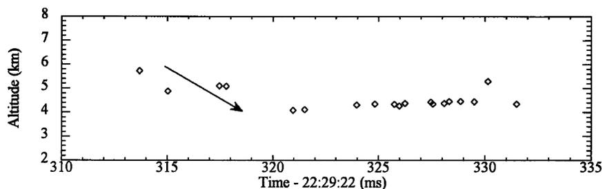
FIG. 9. LMA plot for the CG flash seen in Fig. 7. The arrow indicates the direction of negative polarity breakdown. The movement of negative charge to lower altitudes indicates an upward-pointing  $z$  component of the electric field vector. This is confirmed by the balloon sounding (Fig. 7) measuring an electric field near the flash-initiation location of  $186 \text{ kV m}^{-1}$ .
