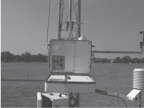
FIG. 6. Portable reference system (center of picture) used by the Oklahoma Mesonet to verify field performance of various sensors. The system is mounted temporarily at the station during the site pass and records measurements of air temperature, relative humidity, solar radiation, and pressure while the technician completes maintenance activities.
