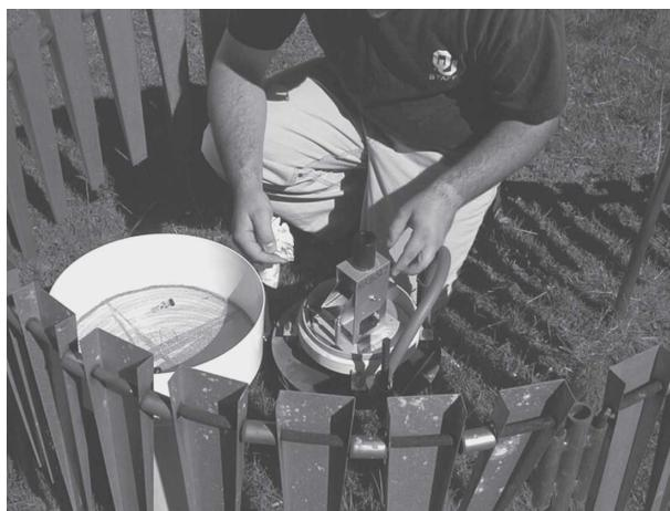
FIG. 5. An Oklahoma Mesonet technician cleans the rain gauge after the initial drip test.
