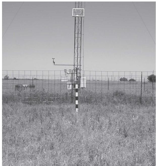
FIG. 7. One of 14 standard digital photographs taken during a site pass at an Oklahoma Mesonet station. The vegetation gauge (striped pole in foreground) indicates the height of the vegetation surrounding the station. The fence outlines a 10 m × 10 m plot, and the tower is centered within this square.
