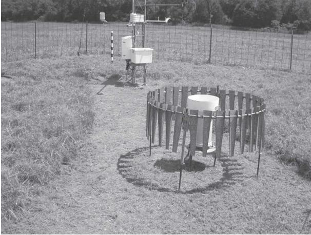
FIG. 3. Example of the vegetation cut for a firebreak around the rain gauge and instrument tower of the Oklahoma Mesonet.
