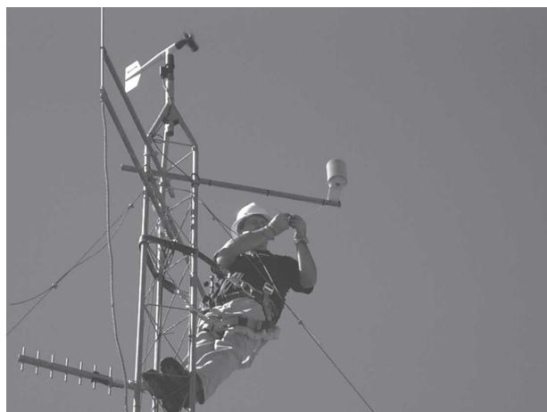
FIG. 4. An Oklahoma Mesonet technician inspects and cleans sensors at the 9-m level.
