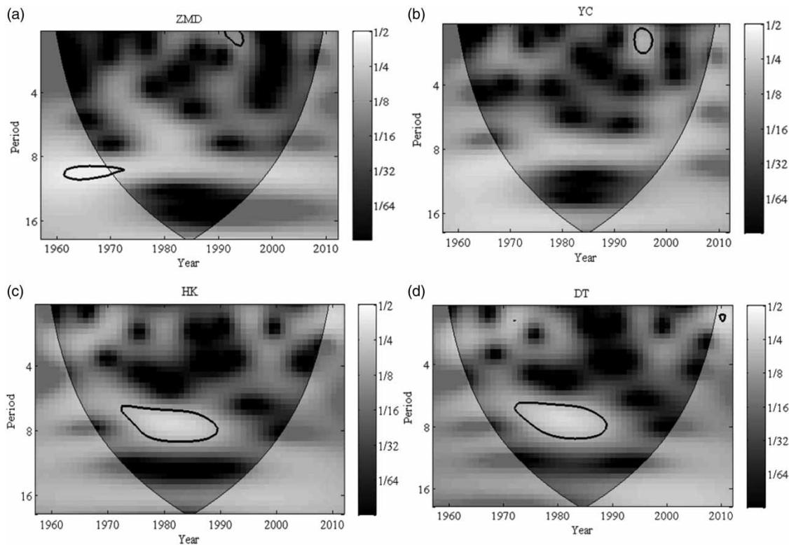
**Figure 2** | Wavelet power spectra of summertime runoff in the Yangtze River basin during 1957–2012: (a) Zhimenda hydrological station; (b) Yichang hydrological station; (c) Hankou hydrological station; and (d) Datong hydrological station.
