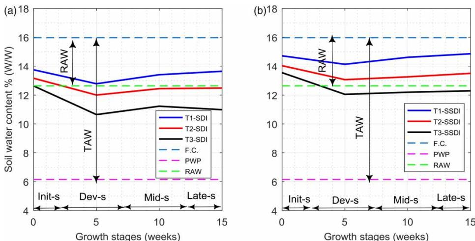
**Figure 5** | Average values of soil moisture content under different irrigation strategies (T1 = 100%; T2 = 80%; and T3 = 60% of crop evapotranspiration) for surface (SDI) and subsurface irrigation (SSDI) systems during the growth stages of the tomato crops. SMC, soil moisture content; FC, field capacity; RAW, readily available water; TAW, total available water; and PWP, permanent wilting point.
