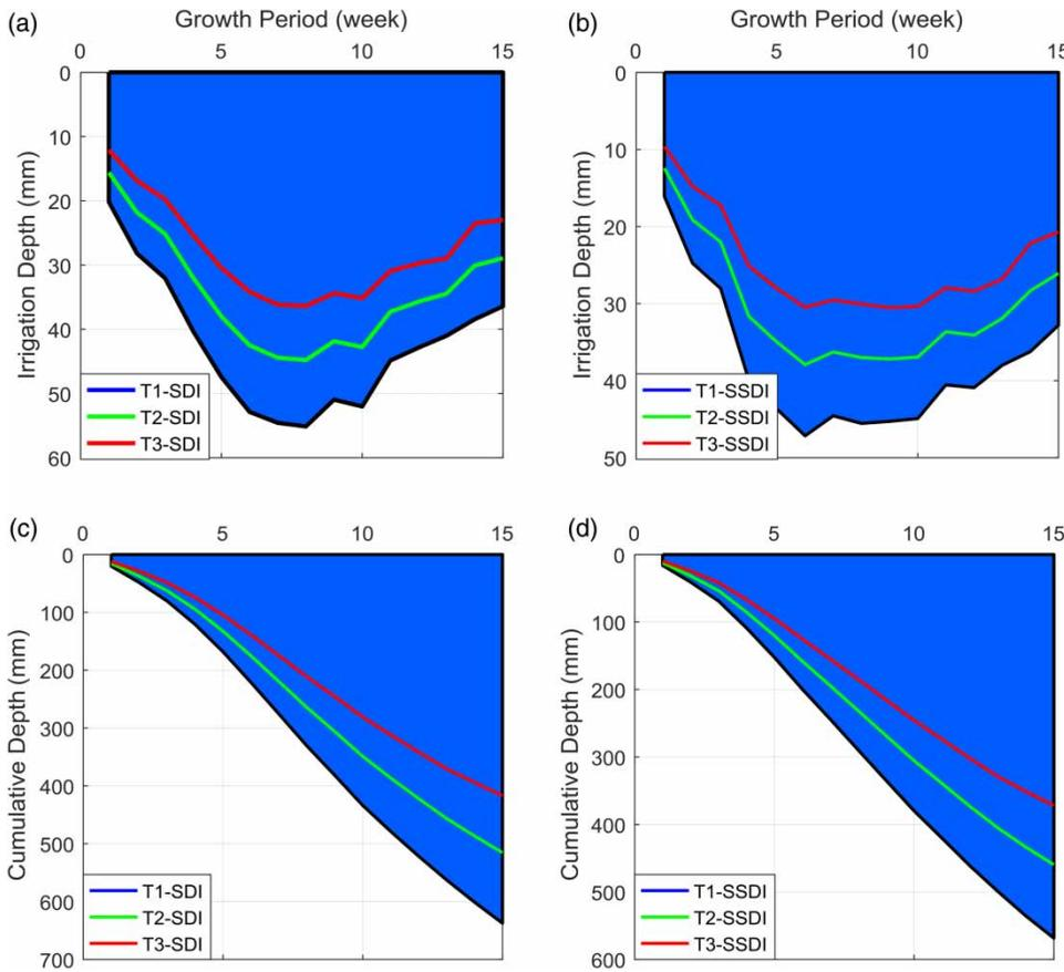
**Figure 6** | Average amounts of water applied under different irrigation treatments (T1 = 100%; T2 = 80%; and T3 = 60% of crop evapotranspiration) using the surface (SDI) and subsurface drip irrigation (SSDI) systems.
