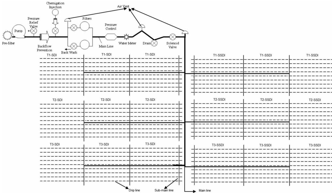
**Figure 3** | Schematic of the experimental field for two types of irrigation methods (SDI and SSDI) and three irrigation regimes: T1 (full irrigation supply), T2 (80% of full irrigation supply), and T3 (60% of full irrigation supply).
