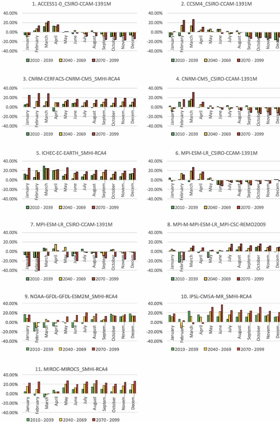
Figure 5 | Predicted change in future mean monthly discharge of Brahmaputra River at Bahadurabad station under RCP8.5 of different RCMs.
