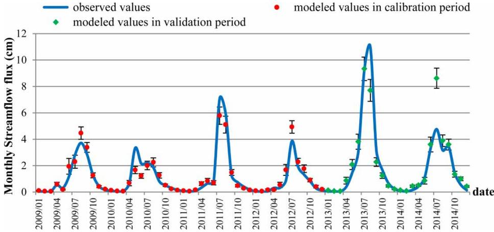
**Figure 3** Time series of observed and modeled monthly streamflow during the research period. The modelled values were the mean value of the posterior samples and the bars denoted the standard deviation.
