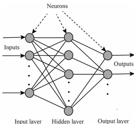
**Figure 1** | A feed-forward artificial neural network structure.
