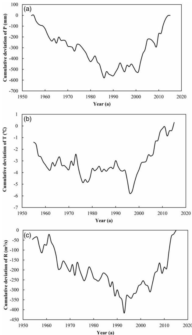
**Figure 3** | Cumulative deviations in precipitation (a), air temperature (b) and runoff (c) based on monthly observations at Kaqun station. Annual precipitation, mean annual temperature and mean annual runoff are denoted by P, T and R, respectively, in Figure 3.
