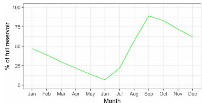
Figure 4 | Reservoir operational scheduling curve developed for the future inflow. The curve is developed using inflow from the ensemble mean of models, and it is the technique used to modify the current operational scheduling.
