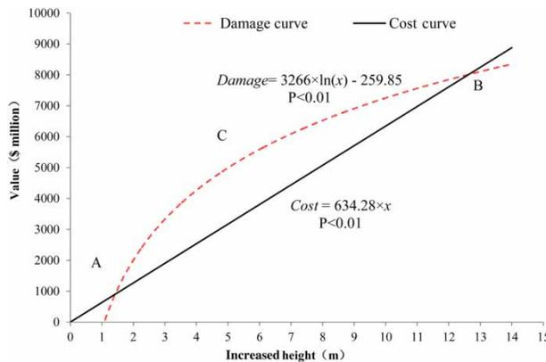
**Figure 4** | The benefit–cost model for dike heightening (the benefit of dike construction is the difference between the damage curve of extreme events (dotted line) and the cost curve of dike heightening (solid line)).
