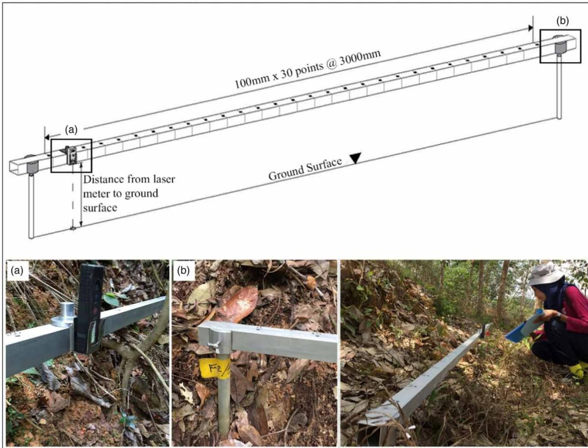
**Figure 3** | Modified Laser Erosion Bridge (a) Laser meter with holder and (b) Connector (Mohamad *et al.* 2018).
