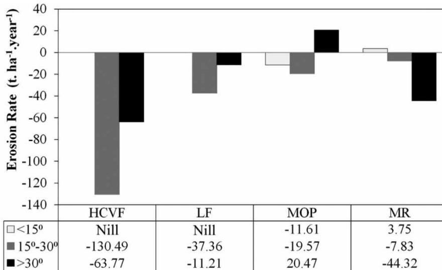
**Figure 8** | Mean erosion rate within three slope classes; <15°, 15°–30°, >30° in different land-use types.
