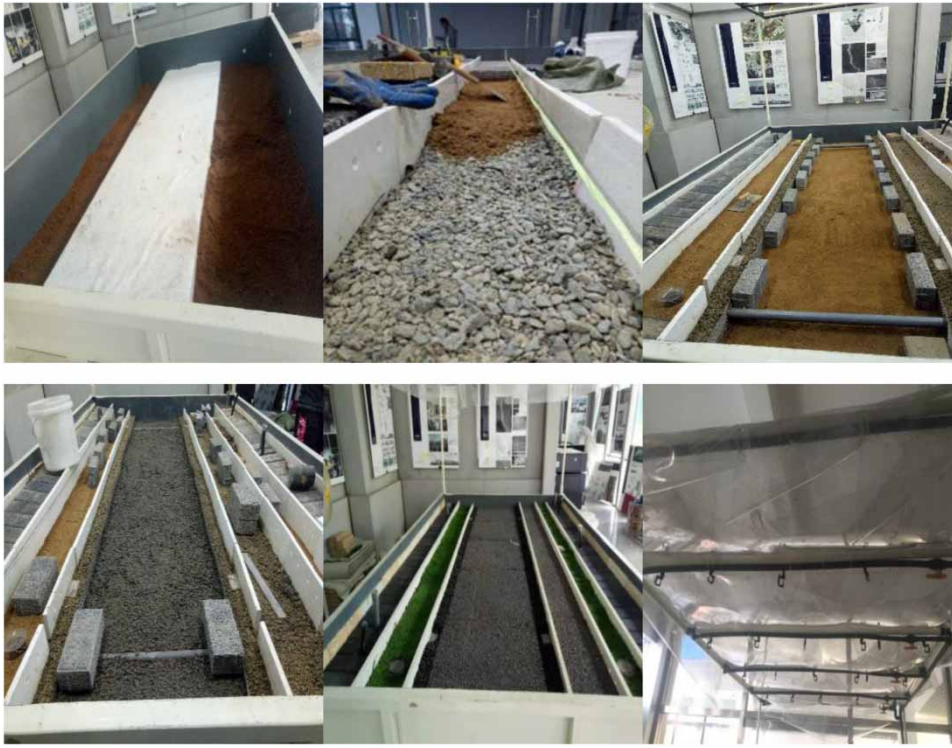
Figure 6 | Rainfall device and scale model.
