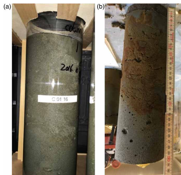
Figure 3 | (a) The column run at 5 °C a few weeks after the leaching experiment had started and (b) the same column at the end of the leaching experiment (taken out of the acryl-plastic column). The column has a 2 cm layer of sludge material on top.
