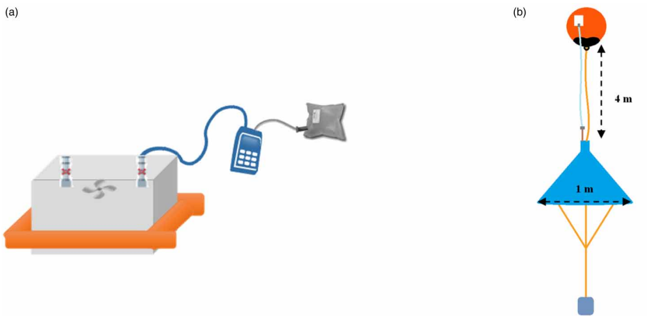
Figure 2 | Determination of emissions. (a) Floating static chamber. (b) Inverted funnel for bubble measurement.
